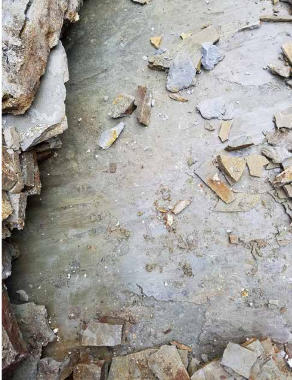
Figure 1. Slickensided remolded clay on a hard siltstone bed at the base of a backcut failure headscarp during buttress excavation.
